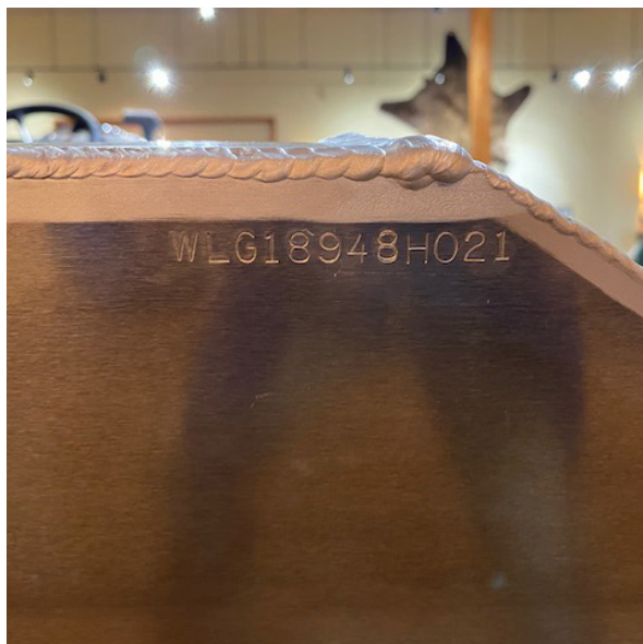
A properly formatted HIN in the proper location at the top of the transom, starboard side
