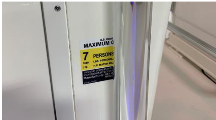
FIGURE 5 Incorrect Example of Capacity Label Placement
