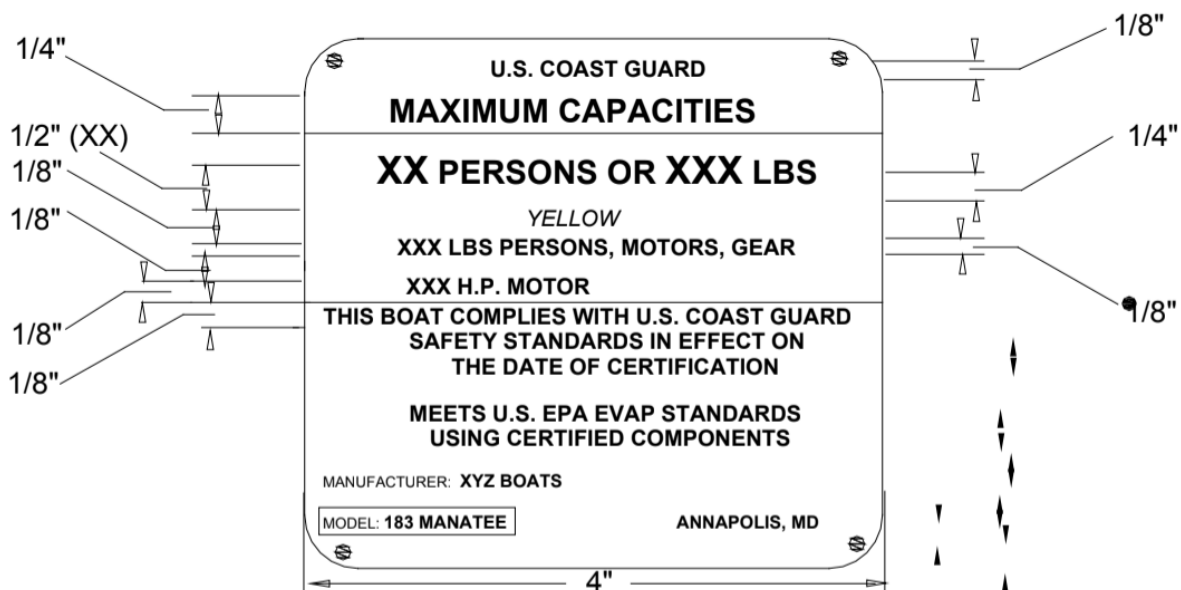
FIGURE 1 Combined USCG Capacity & Certification Label with EPA Statement
